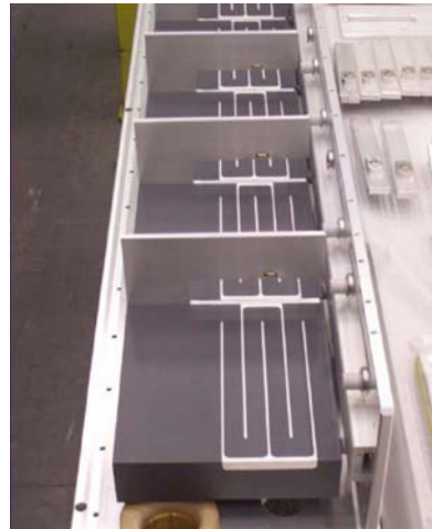
Figure 10: Printed conducting strips directly on top of the ferrite of the MKE-L10 kicker.
