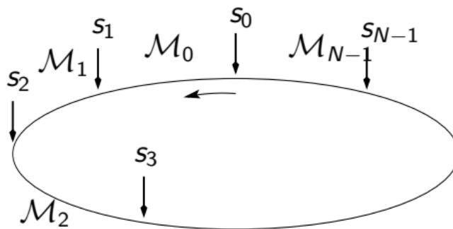
Reading the TWISS parameters  $\psi, \beta, \alpha$  and the positions  $s$  of the elements and building up the matrices for the different points
